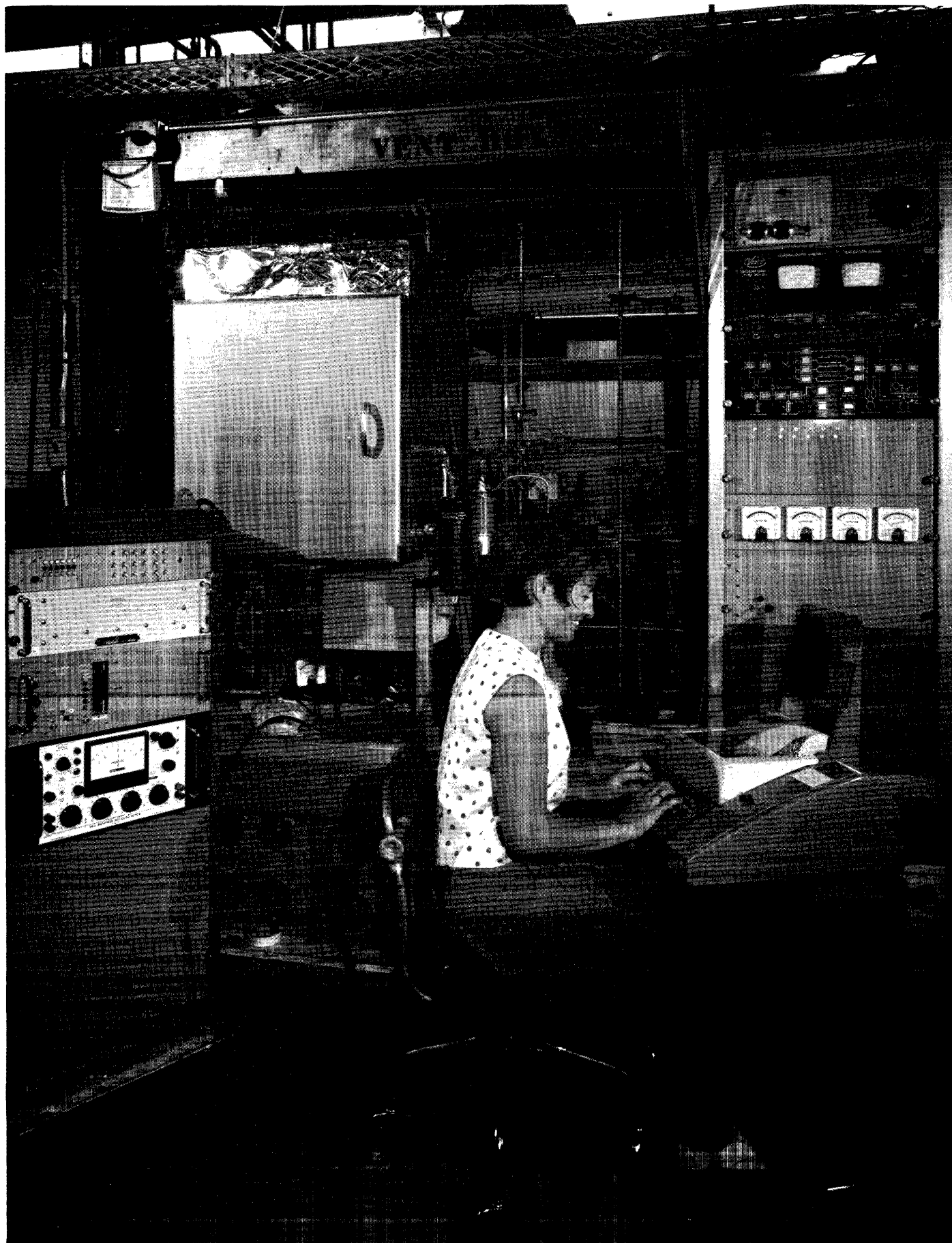
Figure 2 Automated Apparatus Used for the Simultaneous Determination of Carbon, Hydrogen and Nitrogen in Organic Compounds
