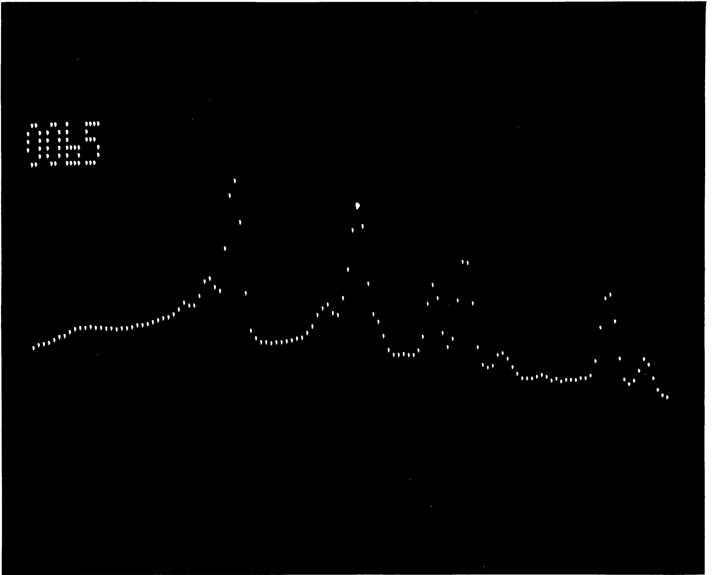
Figure 1 Oscilloscope display of a portion of a 4096 channel gamma-ray spectrum and a number indicating channel position of bright dot.
